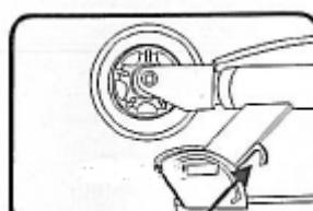
2. Pull the lever upwards.
